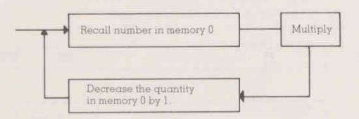
If the first number placed in memory 0 is 17, then the first time around the loop would produce 17 [X], and the quantity in memory 0 would be reduced to 16. After the next loop you would have 17 [X] 16 [X], and 15 would be stored in memory 0. This loop would continue to generate the required series for the factorial.
