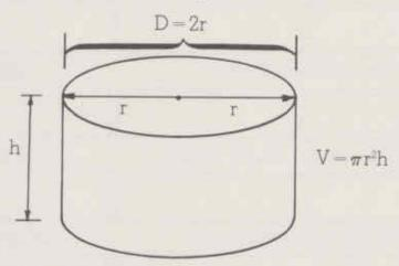
A key point here is that you have to enter two measurements into the formula. You must enter the diameter, D (from that you'll calculate r = D/2), and you must enter the height, h, to finish the calculation  $V = \pi r^2 h$ ).
