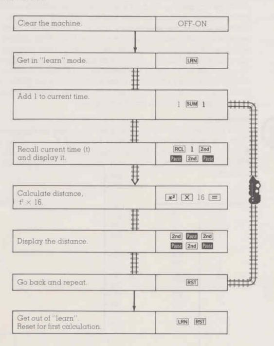
At this point you'd be all set to either write down time and distance in a table as shown on the next page, or graph them right on a graph. As we've mentioned — if the machine starts getting ahead of you, just stop things with the R/S key.
