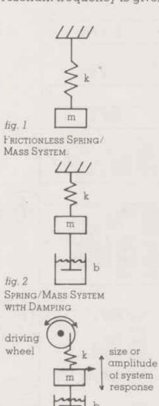
Damped Spring/Mass System with Periodic "Driving Force"
