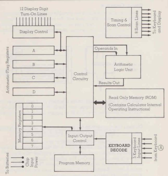
Figure 4: SIMPLIFIED CALCULATOR IC BLOCK DIAGRAM
