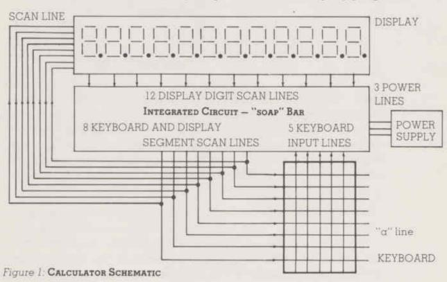
Figure 1 is a simplified schematic diagram of the inside of your calculator, showing the Display, the "SOAP" bar, the Keyboard and the Power Supply. A remarkable thing about the SOAP bar is that for all its power, it's connected to the outside world by only 30 connections. If you consider all of the things the chip has to handle, and all of the information it processes, 30 connections is really a very small number. Let's briefly examine how this works.
