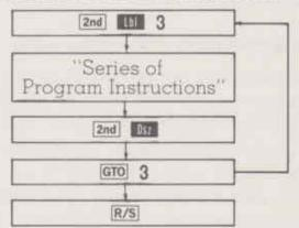
The number of times the "instructions" were executed would be controlled by the number stored in memory zero (stored before running the program). If a 6 were stored in memory zero, the series of instructions would be carried out 6 times, then the program would halt.
