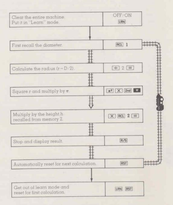
To run this program, just key it in carefully from the flow diagram, then:
