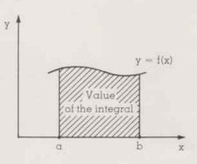
When using Simpson's approximation (or Simpson's rule, as it's often called), you divide the area under the curve into an even number of parts (n). The width of each part, w, is then given by:  $w = \frac{b-n}{n}$ . In the figure shown, we've divided the area into 6 parts, so  $w = \frac{b-n}{n}$ . To compute the approximate total area under the curve (the approximate value of the integral), you use the following formula:
