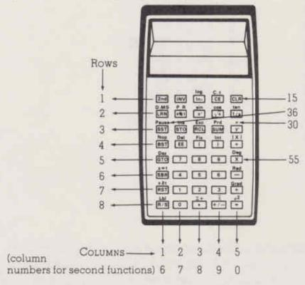
There are 8 rows of keys (numbered 1 to 8 top to bottom), and 5 columns of keys (numbered 1 to 5 left to right.). The key code for any first function key is a two-digit number: the first digit is the row the key is in, the second digit is the column it's in.
