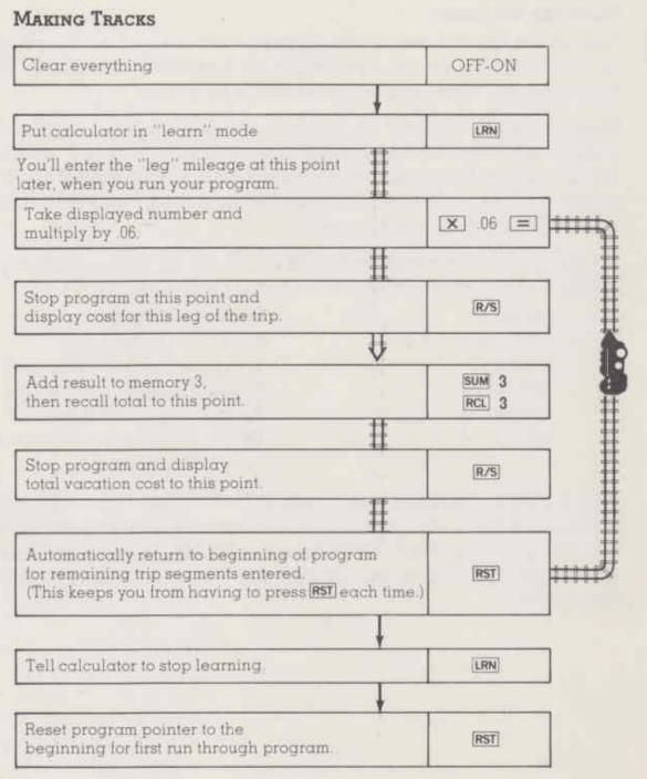
You can key your program in, right from the flow chart, after you turn your calculator OFF and ON. (This important step clears the entire machine and will prevent left over keystrokes from previous examples causing any trouble in this one.)
