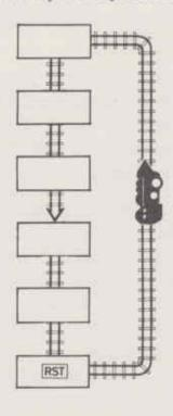
By placing RST at the end of a series of operations, with no R/S as part of the program, you create a continuous "looping" program.
