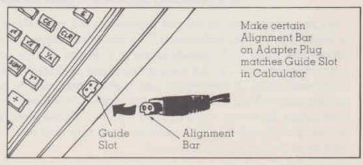
When the battery pack is fully charged, the calculator will operate approximately 2 to 3 hours before recharging is necessary. However, don't hestitate to connect the adapter/charger if you know or suspect the battery pack is nearly discharged. A battery pack near discharge can adversely affect all calculator operations giving erroneous results. A discharged battery pack is typically indicated by a dim, erratic or blank display.
