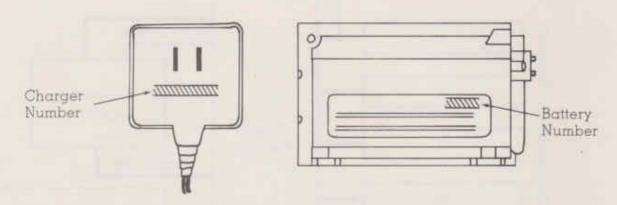
Note: Two different combinations of battery pack and adapter/charger may be used with your calculator. The BP/6 battery pack is used with the AC9131 adapter/charger. The BP/7 battery pack is used with the AC9132 adapter/charger.
