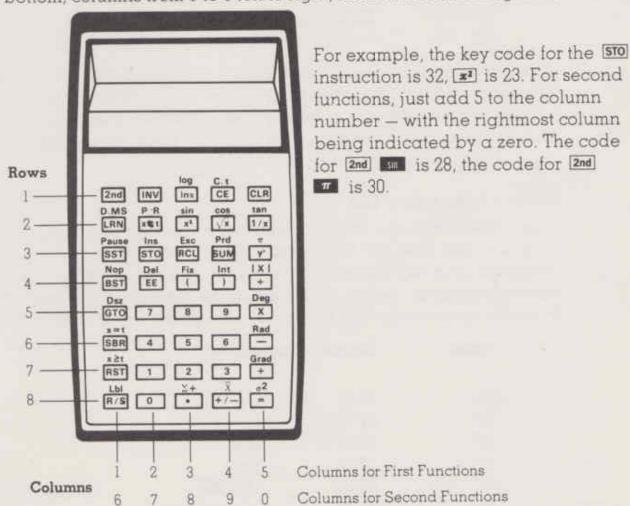
When you first enter a program in "learn" mode, you won't see the key codes, because the program memory display always moves ahead to the next step. To see the codes in any program, you need to enter the program first, then go back and examine the codes. Here's how to do this:
