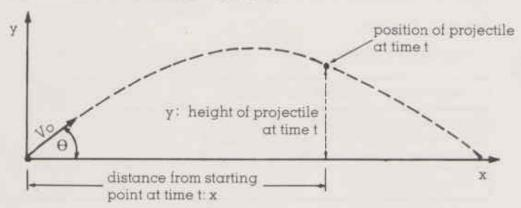
In the case of a golf ball (etc.) projected into the air with an initial speed Vo, at an angle  $\Theta$  with respect to the x axis, the motion would appear as shown above. Once the ball is in the air, the only force acting on it is gravity, which accelerates it downward at g=-9.8 meters/second<sup>2</sup>. The equations which describe how the distance from the starting point (x), and the height off the ground (y) vary with time as the ball flies through space are:
